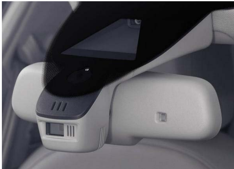
Figure 1.1: A modern ADAS with a camera integrated on the rear view mirror
