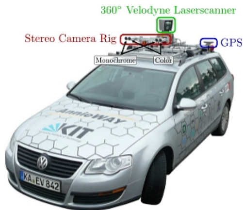
Figure 12: Vehicle used to collect KITTI dataset
