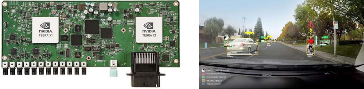
Figure 10: Left: NVIDIA Drive-PX. Right: Obstacle detection demo at CES 2015
