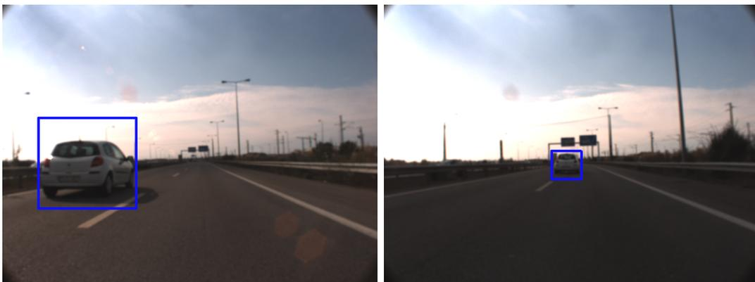
Figure 5.9: Example of near (left) and far (right) car with dynamic bounding box size
