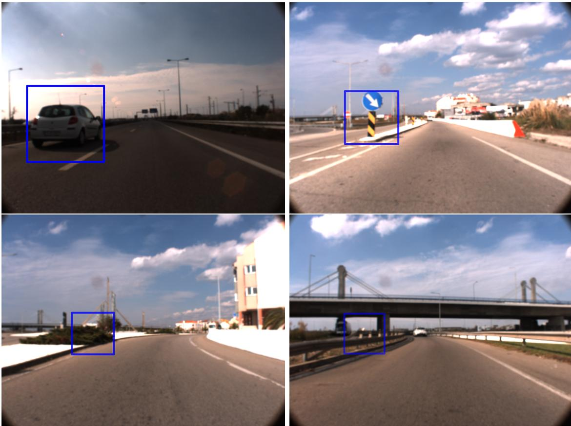
Figure 6.3: Targets acquired using the MTT labelled as `car` (top-left), `sign` (top-right), `misc` (bottom-left) and `DontCare` (bottom-right)
