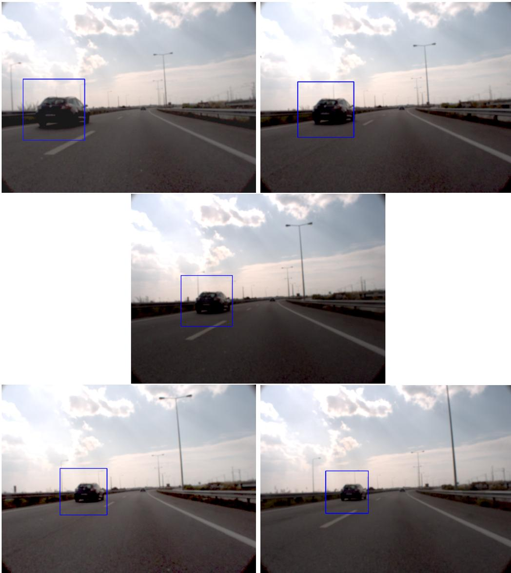
Figure 5.4: Example of back tracking and front tracking: the picture in the middle is the selected frame, the two upper frames show the back tracking and the two lower frames show to front tracking.
