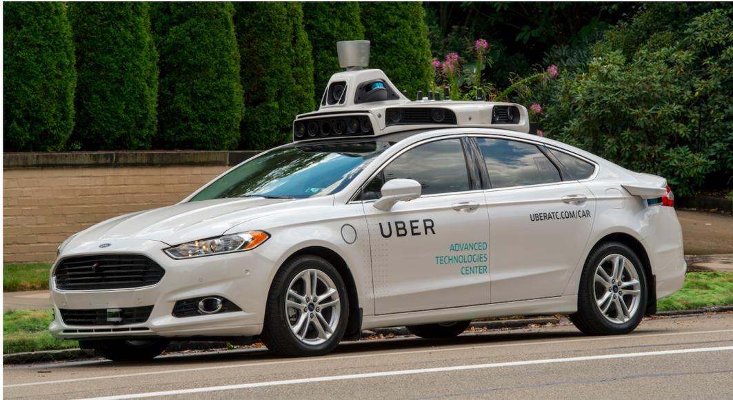
Figure 2.3: Ford Fusion Uber ATC car (Uber Advanced Technologies Group 2018)
