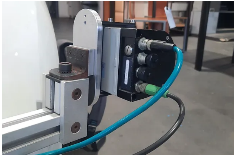
Figure 4.2: LIDAR with new supports applied.
