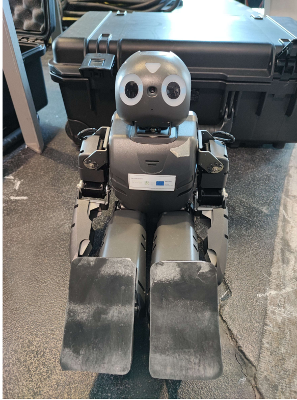
Figure 5.1: Picture of the Darwin-OP with the neoprene rubber feet.
