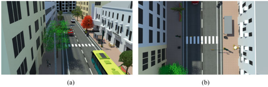
Fig. 6.2 Example of inverse perspective mapping from a oblique view; into b top view
