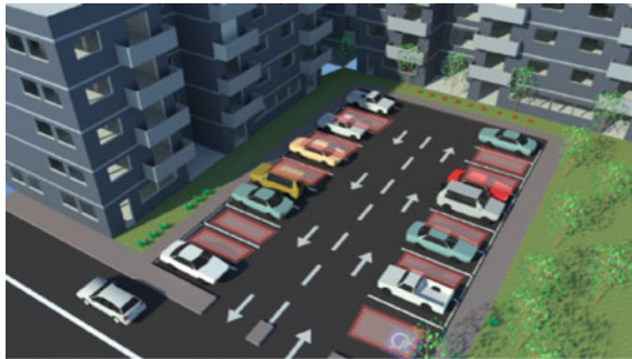
Fig. 6.3 Illustration of parking space detection in a parking lot (10 free space highlighted in red box)
