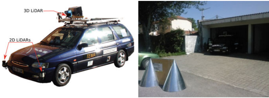
Fig. 7.2 ATLASCAR1 and the LiDAR sensors on-board (left). Conic calibration target (right)
