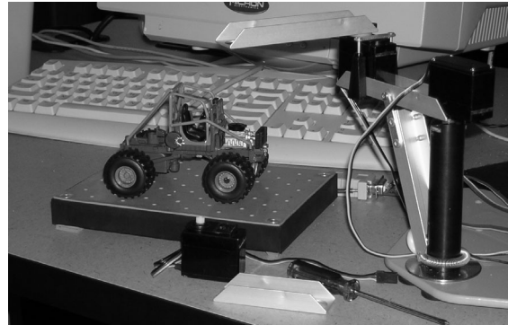
Figure 1 A partially assembled Robix RCS-6 manipulator for “spot welding” laboratory exercise.
