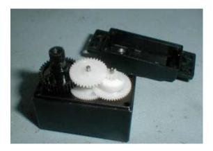
10. Assuming that the gear didn't come off already, remove it carefully and set aside. Remember that it has grease on it, so set it down somewhere clean. Dirt or anything else will stick to it and can cause damage when the motor is spinning later. So keep that and all the other gears clean.
