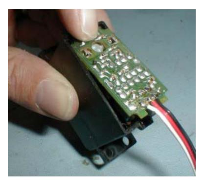
13. Once you have reassembled the motor, test it using the DARC Board or some other device that will generate the proper signals to drive it. If it works in both directions okay, you're done. If not, you may have to disassemble it and repair some work that was done incorrectly.
