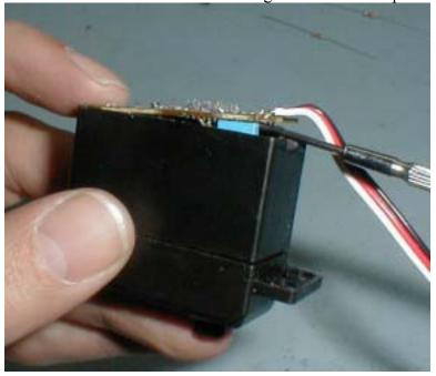
4. Remove the potentiometer from the case. The pot will have 3 leads similar to that shown. For a model other than the Futaba S3003 the leads may be wires instead. Either way, the pot will go up into the body of the motor, inserting into the output gear above. Gently remove the pot. You should hang onto it in case you want to restore the motor to partial rotation. You may also be able to use it in a circuit later.
