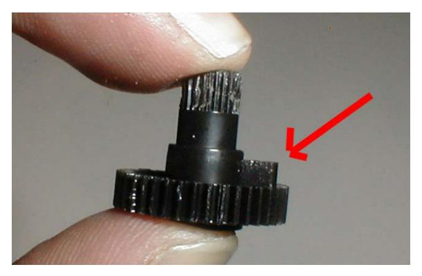
You can use a pair of snippers to carefully nip off pieces of this stop. Start at the outside and snip off small pieces at a time rather than trying to get it all in one cut. If you try it in one, you may break the gear, ruining the motor. If you have a rotary cutting tool, use it instead of snipping.
