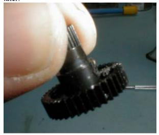
12. Replace the gears and the top cover. Refer to the beginning photo if you don't remember what gear goes where. Then put in the circuit board. Be sure that the cable rests in the recess so that the bottom cover will go on flat.
