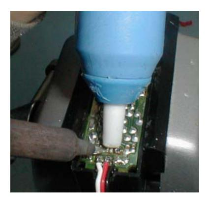
3. VERY CAREFULLY, lift out the circuit board. Once you have desoldered the motor connections and the pot leads, it should come out pretty easily. You may need to apply GENTLE pressure with a small screwdriver or similar device to get it started. But if it takes more than slight pressure, then recheck your desoldering work. Most likely you still have some solder which is holding the board to the parts beneath.
