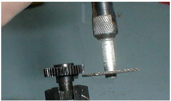
Again, you must be careful. Not just of trimming your fingers but also of trimming the teeth on the gear. You also want to be careful not to throw dust onto the motor's other gears below you if you have it sitting on the bench where you are using the rotary tool.
