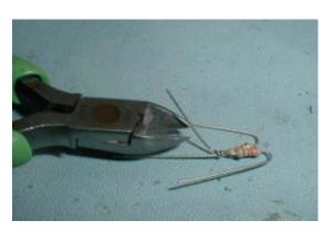
7. Place the combined resistors into the holes where the pot leads went. The lead where the two resistors are joined must be in the middle hole. Otherwise what lead goes where does not matter.
