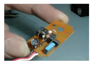
8. Solder the resistor leads in place and snip off the excess.
