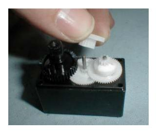
11. Remove the output gear, which is usually black as shown in this photo. It will have a mechanical stop on it which will prevent the motor from rotating more than 180 degrees, so you must remove this stop in addition to the potentiometer replacement.
