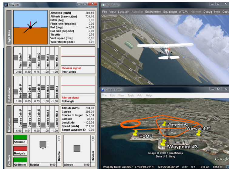
Figure 1.7: Uavplayground project, a GUI with GPS tracking waypoint and circling navigation [24].
