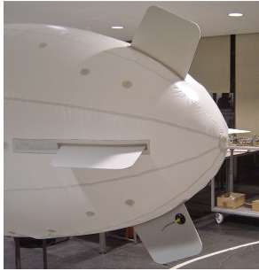
(a) Rear stabilizers, and the rear thruster positioning in detail.
