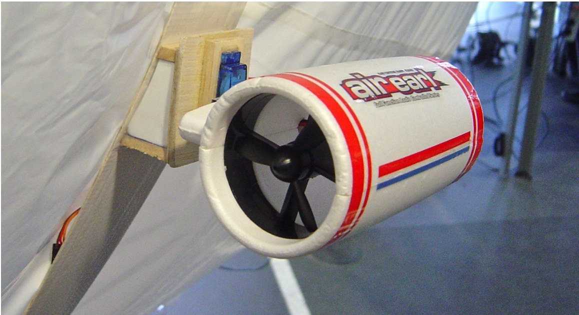
Figure 3.4: Render of the ducted fan based propulsion system developed.
