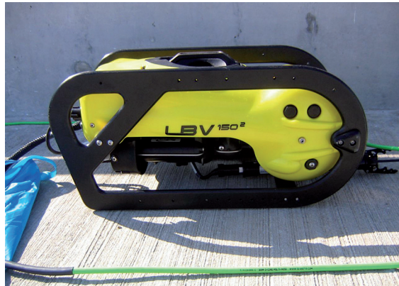
Fig. 50.5 A small UUV used for underwater inspection (courtesy of CRASAR)
