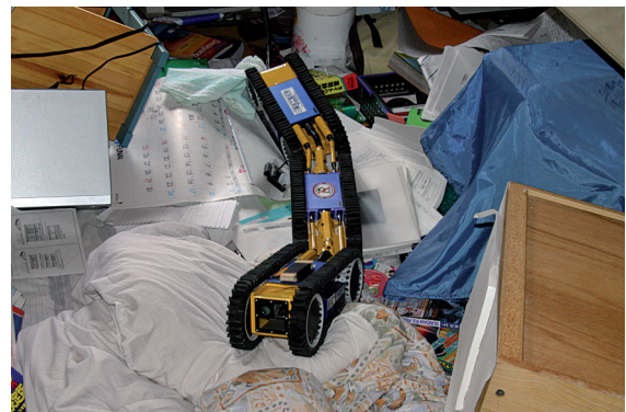
Fig. 50.3 IRS Soryu robot searching a house destroyed by the Niigata Chuetsu earthquake (courtesy IRS)
