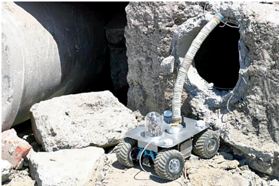
Fig. 50.7 A CMU fixed-base snake being tested at a facility in California (courtesy H. Choset)
