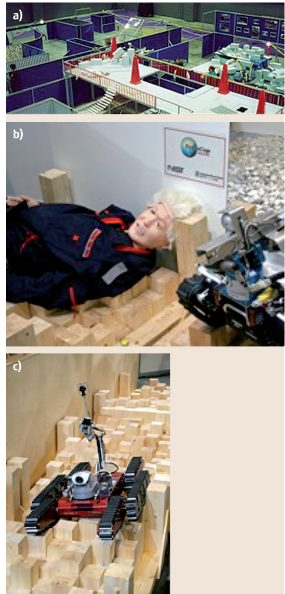
Fig. 50.9a–c View of the NIST standard test bed for search and rescue used by RoboCup Rescue. (a) View of overall test bed, (b) dummy representing a victim, and (c) a step field challenging robot mobility (courtesy NIST)
