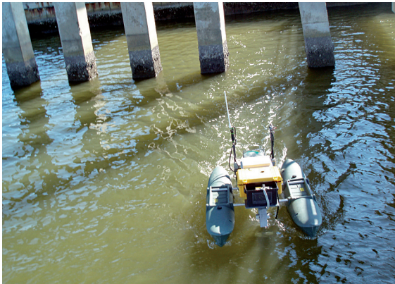
Fig. 50.4 Unmanned surface vehicle exploring the bridge to Marco Island, Florida (courtesy of CRASAR)
