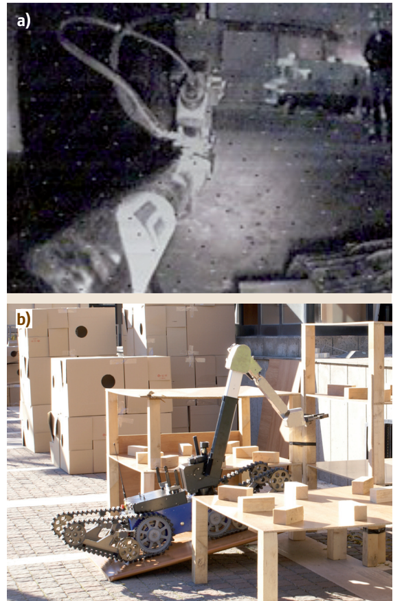
Fig. 50.6a,b Examples of tracked robots with manipulator arms that have been used for disasters or rescue competitions. (a) View from Foster–Miller Talon at the WTC of its arm (courtesy of CRASAR) and (b) telemAX by Telerob at the Rescue Robotics Camp (courtesy of R. Sheh)
