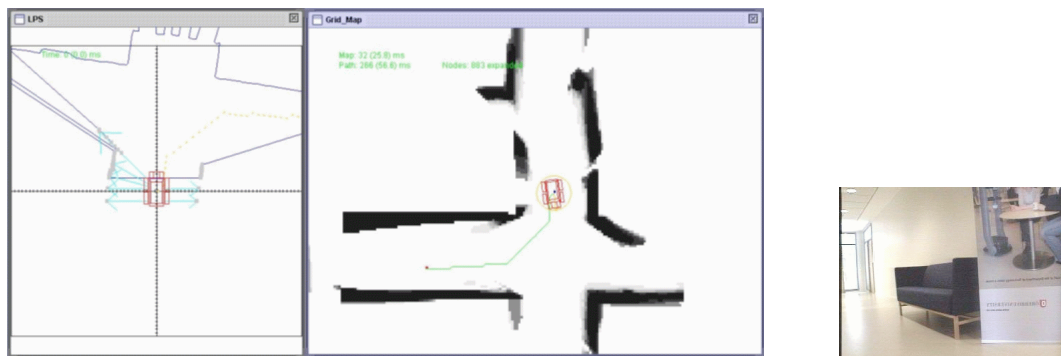
Figure 3.10: The GasBot operator interface. The leftmost window displays the sensor readings in the vicinity of the robot; the middle window displays the current environment map built by the robot; the rightmost window shows the images taken by the robot camera.
