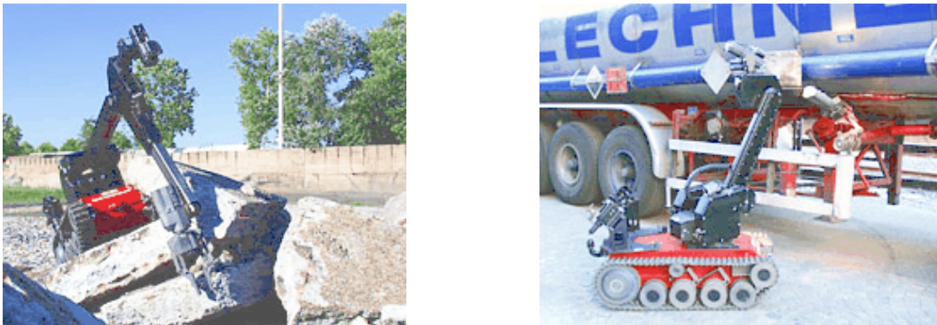
Figure 2.10: The Safety Guard variant of the tEODor robot built by IPA/BASF, performing two different tasks involving hazardous manipulation
