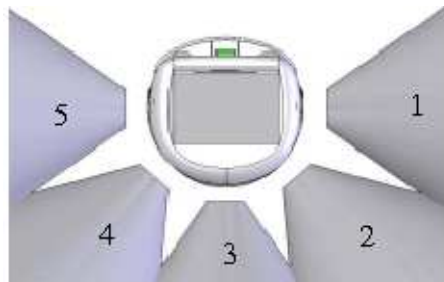
Figure 3.10: Position of the 5 UltraSonic sensors.
