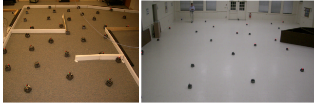
Fig. 3. Left: A dispersion into a small test space used to characterize the performance of different dispersion algorithms. This environment is approximately 6 m x 6 m, with several walls and “rooms”. Right: A dispersion into a large room, note the person in the upper-left corner. It took about 20 minutes for them to achieve this dispersion, but they had to travel through a narrow hallway to get to this space, slowing their progress.
