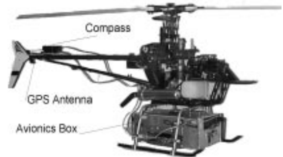
Figure 1. M.I.T. Xcell-60 with avionics system
