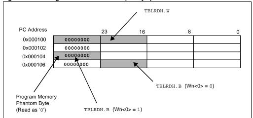
Figure 4-6: Program Data Table Access (MS Byte)
