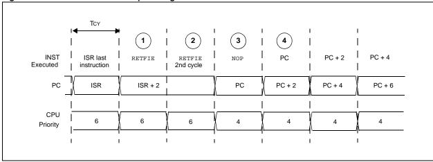
Figure 6-6: Return from Interrupt Timing
