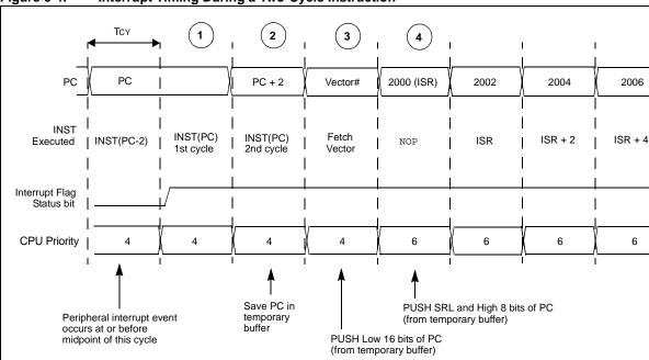
Figure 6-4: Interrupt Timing During a Two-Cycle Instruction
