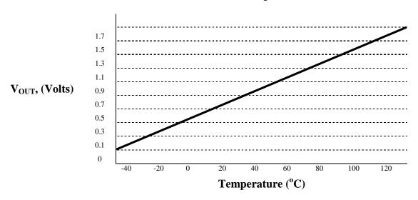
In the units of volts V<sub>OUT</sub> for the TC1047A is given by;
