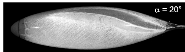
Fig. 2 Limiting streamlines of the inclined bare LOTTE hull [3] ( \alpha=20^\circ , Re_v=3.9 \times 10^5 , fully turbulent flow)
