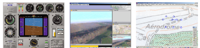
Fig. 6. ReSSAC control screens for “out-of-sight” control, navigation and capture of geo-referenced images.
