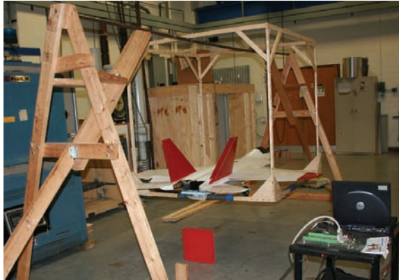
Figure 7 Experimental Setup for Measuring Aircraft Moments of Inertia
