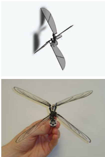
Figure 11. Dragonfly M.A.V prototype
