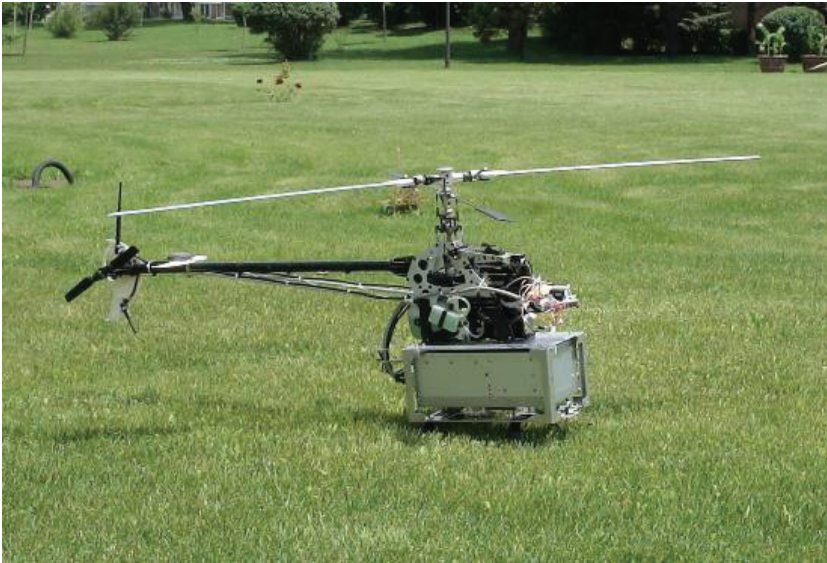
Figure 4. Implemented rotorcraft UAV
