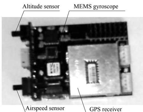
**Fig. 3** Flight control system package
