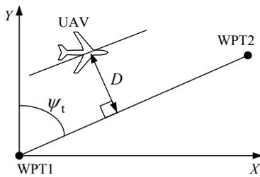
Fig. 7 GPS navigation geometry operation
