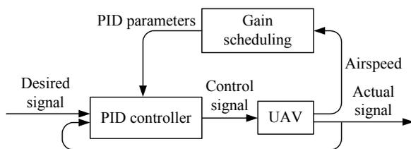
Fig. 8 PID controller using gain scheduling based on the airspeed
