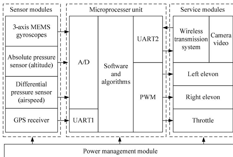
**Fig. 2** Flight control system hardware architecture
