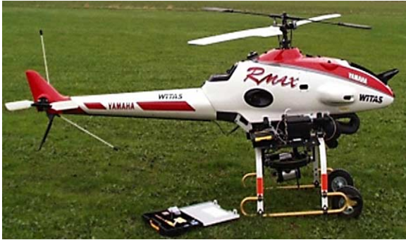
Fig. 4. Yamaha Rmax platform used in the WITAS project.
