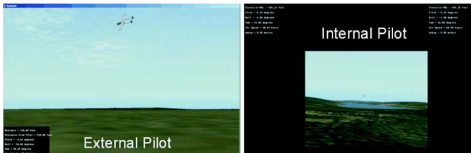
Fig. 4 Simulator screen shots using the Mako UAV model. Left external pilot view point with telemetry data presented on screen. In the real world, this data is normally relayed to the pilot through a headset. Right internal view point with telemetry data presented. The view simulates a nose camera position on the aircraft and replicates the restricted field of view
