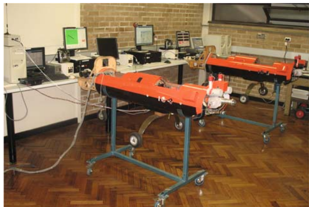
Fig. 17 The HWIL simulation set-up for two Brumby Mk III UAVs
