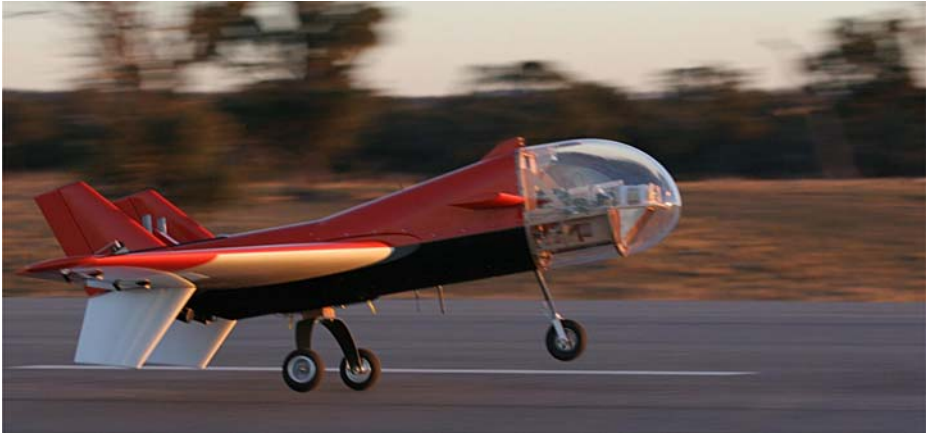
Fig. 2 The Brumby Mk III UAV as it takes off. It has delta wing with 2.9 m wing span, pusher type propulsion, conventional tricycle undercarriage, and replaceable sensor nose cone
