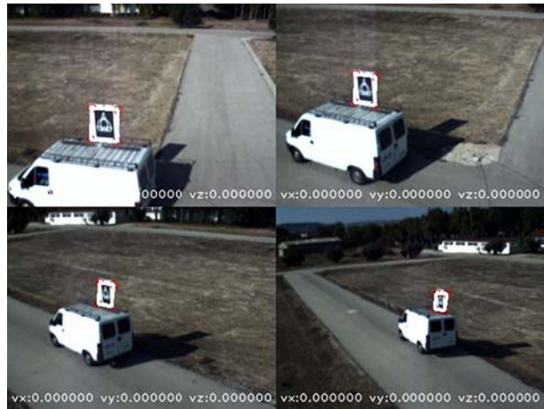
Fig. 14 Tracking of moving object. Servoing is performed on the pan-tilt platform. Notice that velocity in the cartesian coordinates is 0.0 (each component is printed on the image) since the UAV is hovering. Tracking is performed using corner features as explained in Section 3.2
