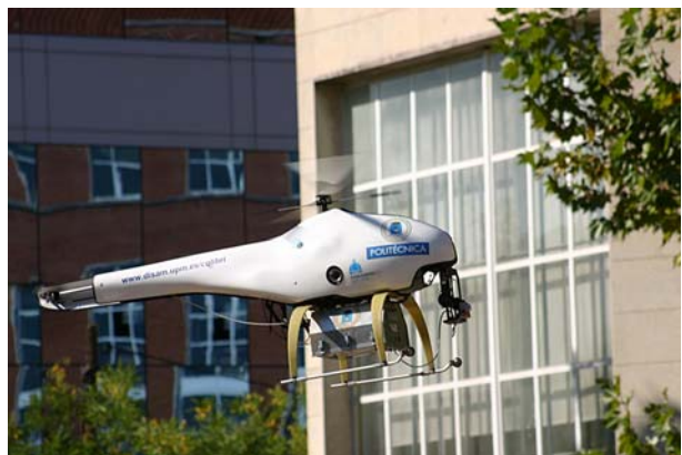
Fig. 1 Aerial platform COLIBRI while is performing an experimental detection and tracking of external visual references
