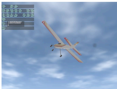
Fig. 8. Hardware in the loop simulator 3D visualization
