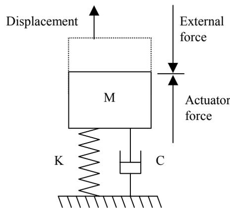
**Figure 2** Impedance control free body diagram
