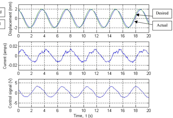
**Figure 6** IPMC sine wave response
