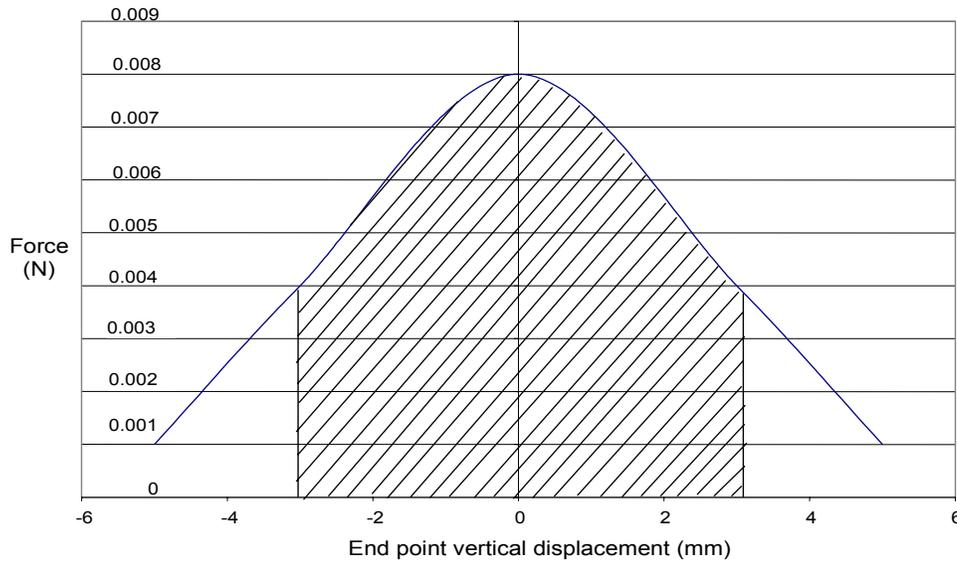
**Figure 3** IPMC force output against endpoint displacement
