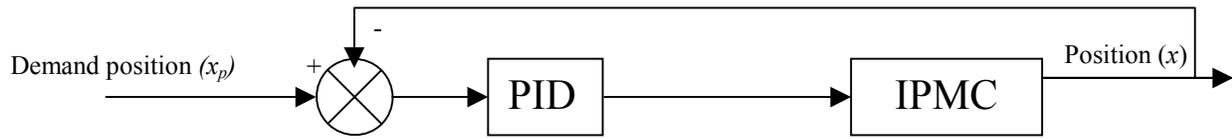
**Figure 4** PID controller
