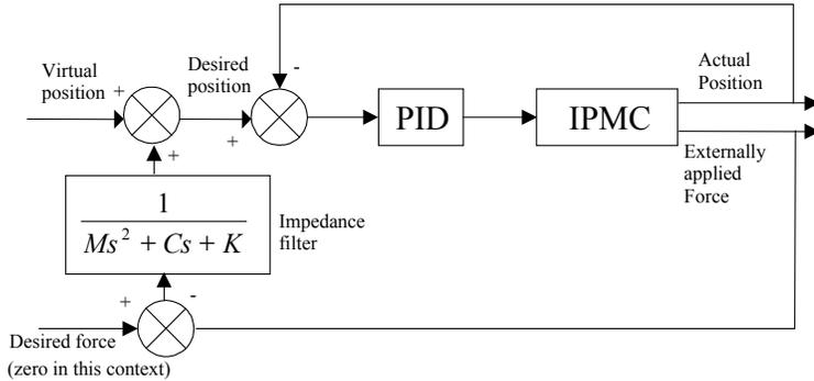
Figure 7 Impedance controller block diagram
