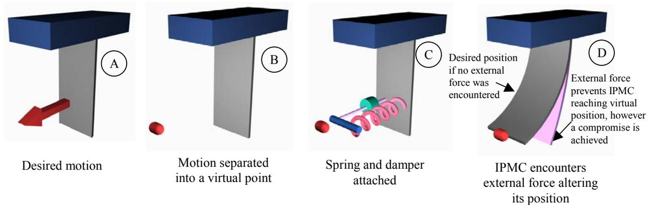
Figure 9 IPMC impedance controller behavior
