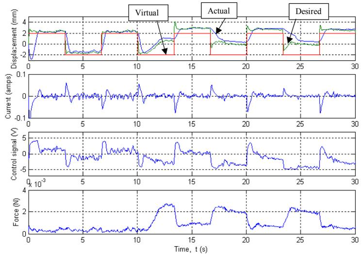
Figure 11 IPMC impedance response ( $K=5$   $C=0.1$ )
