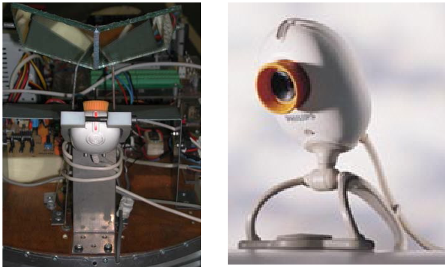
Figura 27 – Webcam Philips Toucam pro.
