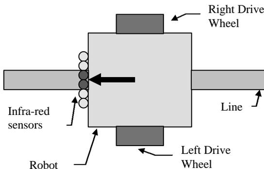
Figure 1 – The Line Following Robot
