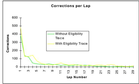
Figure 5 – Number of Corrections needed per Lap
