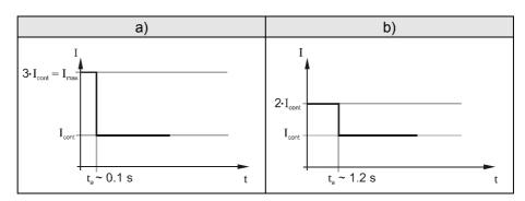
During the time  $t_a^{\ 1}$  a higher current is permitted for motor acceleration. The current is then limited to the continuous output current  $I_{cont}$ .
