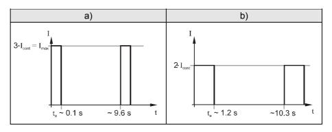
In cyclical mode, the max. output current  $I_{max}$  is available after a break of approx. 10 s, provided that the current between the acceleration processes is zero, otherwise time  $t_a$  is reduced.
