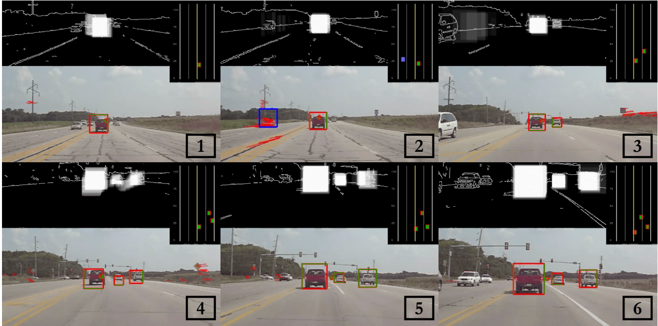
Figure 8: Some of frames that are extracted from the result movie file. Red rectangles show the cars that are detected by the Viola detector. The blue rectangle is the cars that are detected by the optical flow. White area represents the history of detection. That is the area have high probability of cars. Upper right part shows the locations of cars that is mapped onto 3D.
