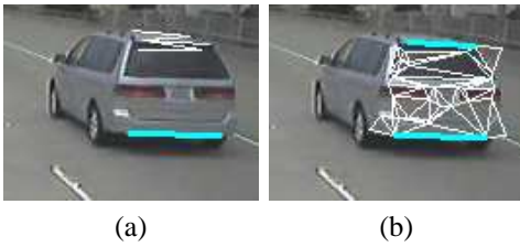
Fig. 2. (a) The top line candidates of an example baseline candidate. (b) A triangle grouping result given two horizontal line segments.
