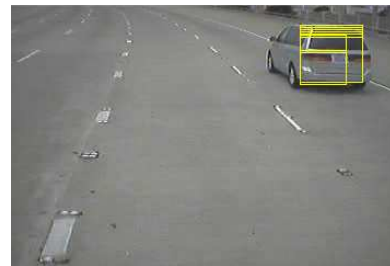
Fig. 5. The selected hypotheses obtained by applying the support vector machine classifier. Among the overlapping hypotheses the largest one is finally chosen.
