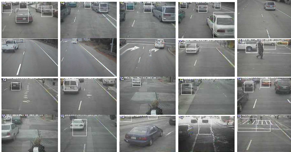
Fig. 6. Example detection results. Both good and bad (in the last row) results are shown.
