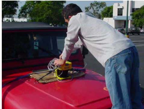
Figure 6-1: Mounting the LIDAR
