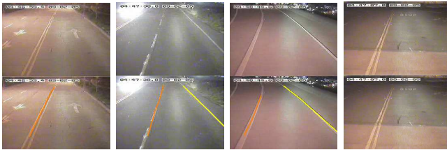
Fig. 10. Example results on images with low illumination. The right most on is a misdetection case.
