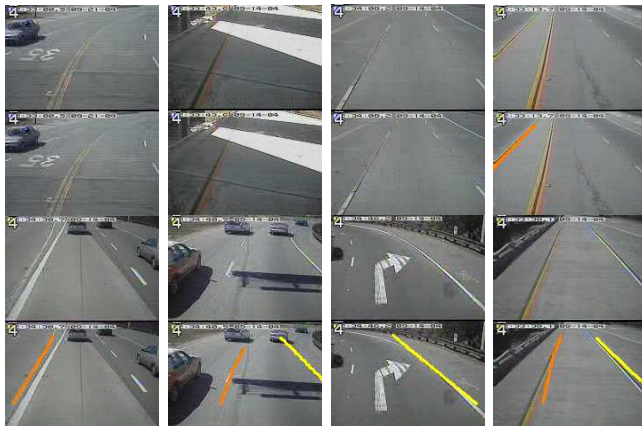
Fig. 9. Example misdetection and false alarms. Only three cases of significant false alarms or tracking failure were reported in two video clips of about 2200 total frames.
