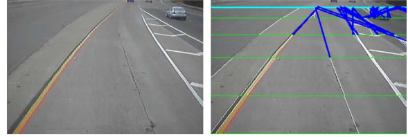
Fig. 10. Horizon detection of the CHEVP algorithm [7] can easily be distracted by ground markings and leading vehicles. In our implementation (for the comparison purpose), we did not use the horizon voting but estimated it from the calibration parameters to get better results.
