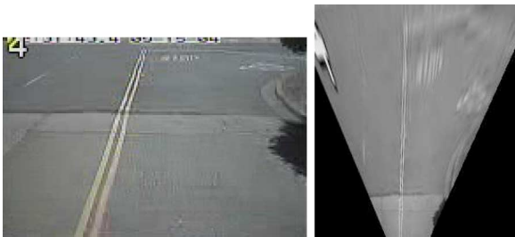
Fig. 3. Example image and a rectified image.
