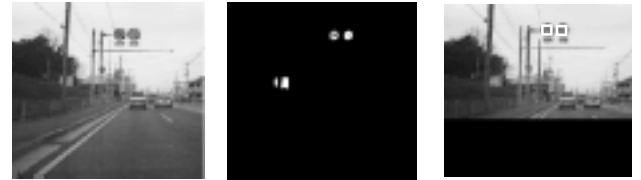
Fig. 4: Detection of speed sign candidates.
