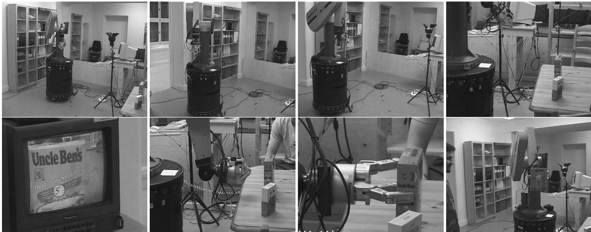
Figure 12: An experiment where the robot moves up to the table, recognizes the rice box, approaches it, picks it up and hands it over to the user.
