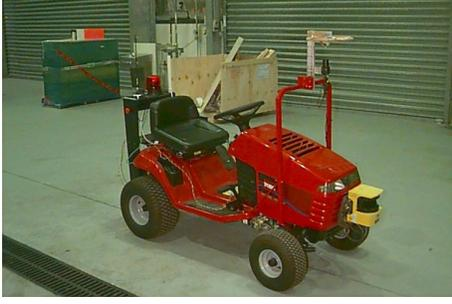
**Figure 10:** The experimental platform. Note the omnidirectional camera mounted over the front wheels and the box at the rear which houses the control and computer system.
