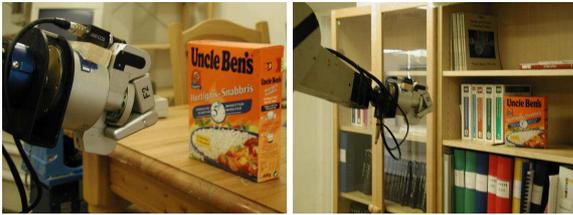
Figure 2: The left image shows the gripper in a reference position while the right image shows the camera in another position and situation. Servoing is then used to move the camera to the reference position relative to the object.
