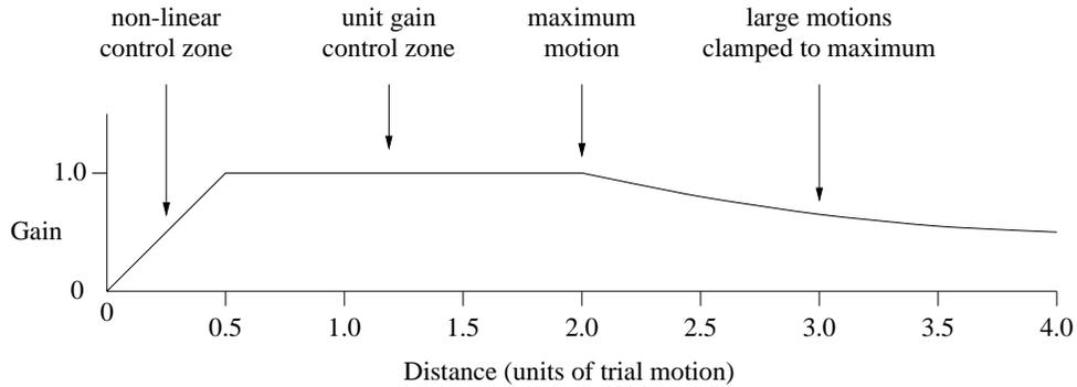
Fig. 11. Gain curve for non-linear control system
