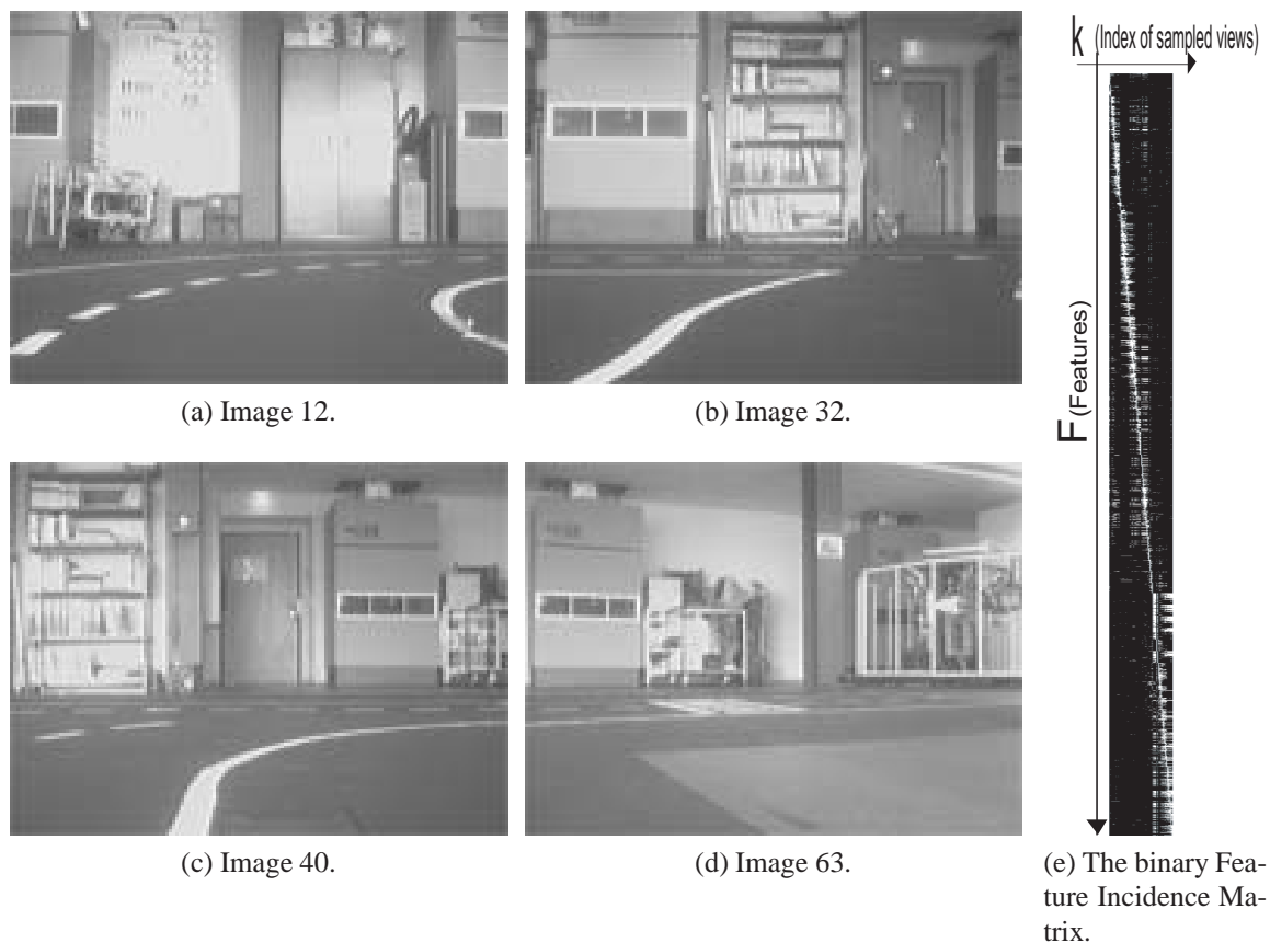
Figure 2.5: Seen here are four representative images from a sequence of sixty seven images taken by Camera #2 as the robot moves inside a large room. The figure at right is the resultant Feature Incidence Matrix, FIM.
