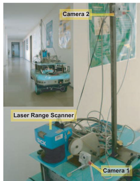
Figure 2.3: Arrangement of sensors on the Robuter mobile robot platform. The sensors used in this work include the forward-facing Camera #1 , the lateral-facing Camera #2 and the LRF mounted on the front of the robot.
