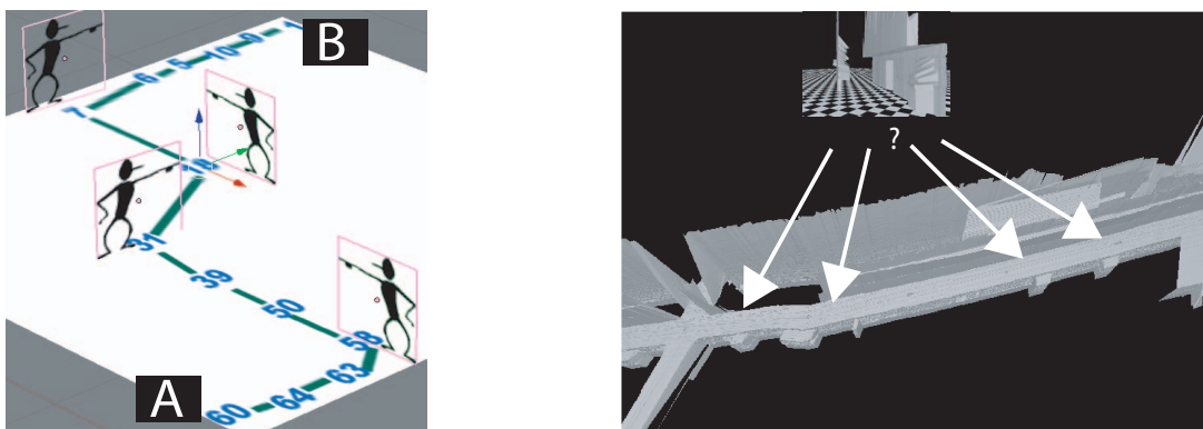
Figure 4.2: The robot is led through the environment on the Environment Familiarisation run, left. The 3D point clouds must be registered in the environment, right.
