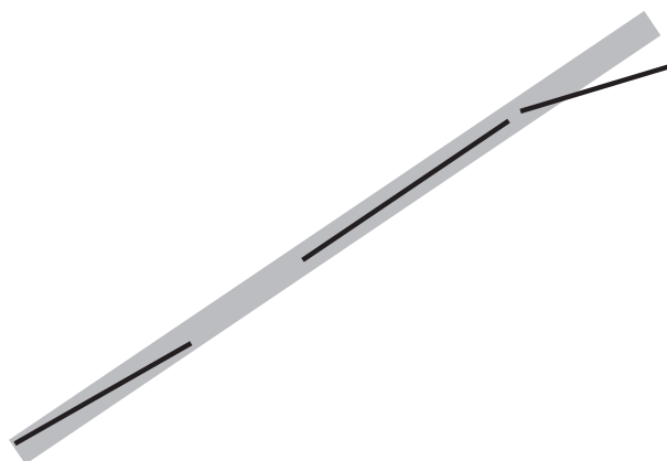
Figure B.1: Two failed attempts at fusing pair of lines are shown. The middle segment cannot be paired with the segment at right because the slopes are quite different (lines within the grey region are eligible for fusion). The middle segment cannot be paired with the segment at left because the two are separated by a large distance.
