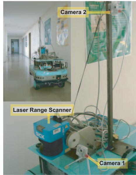
Figure 5.3: Arrangement of sensors on the Robuter mobile robot platform. The sensors used in this work include the forward-facing Camera #1 , the lateral-facing Camera #2 and the LRF mounted on the front of the robot.
