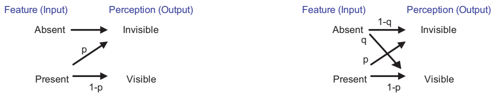
Figure 6.5: Viewing perception as a transmission of a single bit across a noisy, non-symmetric binary channel.
