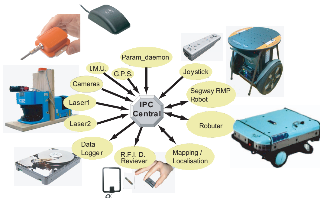
Figure 5.6: Inter-process communication is now performed using CARMEN programming style and the IPC-central application. Shown above is the Laser range Finders, camera and pose sensor mounted upon the Segway RMP robot. All communication is performed using CARMEN.
