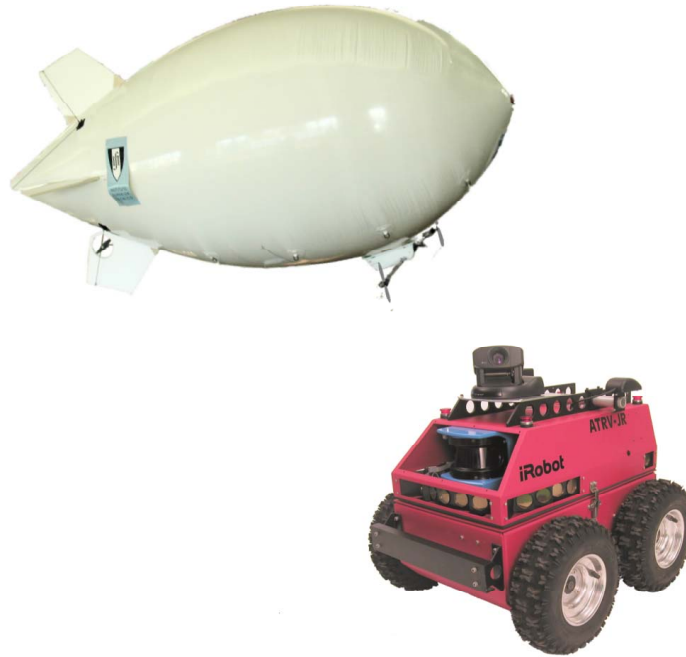
Figure 1.12: The two platforms of the Rescue Project: on the left side the aerial blimp/zeppelin robot and, on the right side, the ATRV-Jr (a land indoor/outdoor robot)
