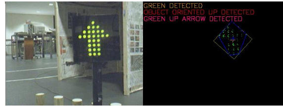
Figure 25 - Traffic lights in 2005(left) and algorithm output (right).
