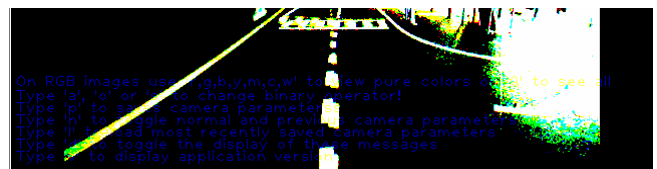
Figure 5 - RGB threshold of merged images in the offline user interface.
