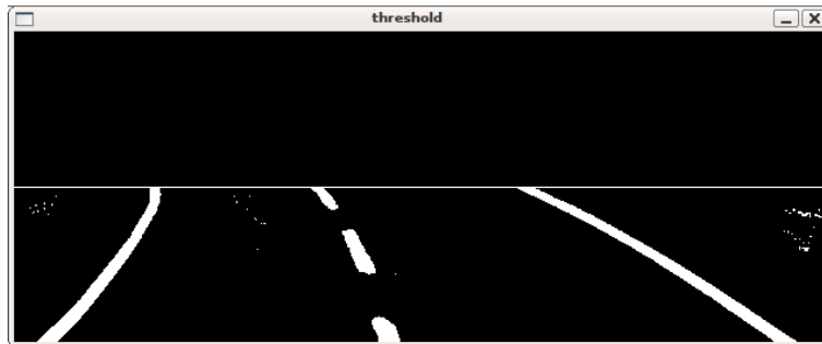
Figure 3.5: Binary road image after an adaptive threshold operation with virtual horizon
