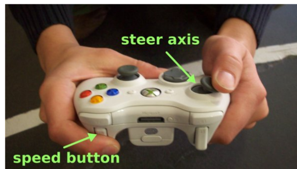
Figure 3.12: Gamepad with steer axis and speed button pointed
