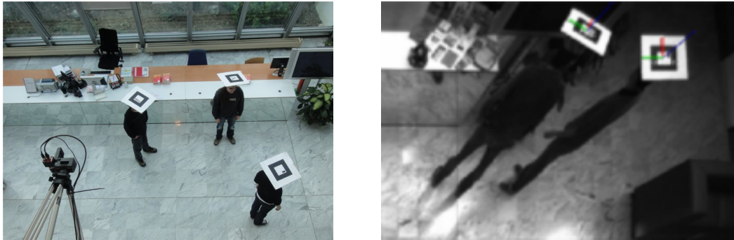
Figure 4.2: (a) Subjects wearing hats with markers and the overhanging camera (left bottom) at INRIA’s hall. (b) Detail of the tracking system showing a three-axis reference system drawn over each marker.
