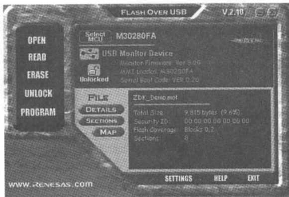
Screen Capture 11.1: The FoUSB window gives us all of the pertinent information about the file that is loaded in its buffer.
