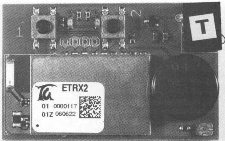
Photo 16.5: Two buttons, two LEDs, a piezo speaker and a light sensor—that's the mix on the MCB. Power for the MCB can be taken from the 4-pin header pins, which also pin out the TX and RX serial connections, or the power connector with the "T" label. The 1.27-mm connection pads are not used and the ETRX2 is mounted directly to the MCB by its solder pads.
