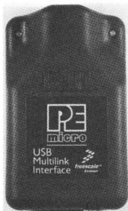
Photo 13.5: This dongle has saved my butt many times during the writing of the Freescale Semiconductor-based chapters of this book. It is reliable and easy to put into play even when you're in the ditch. I like the way the Panasonic PAN802154HAR00 application note puts it: "For serious application the BDM tool is recommended."
