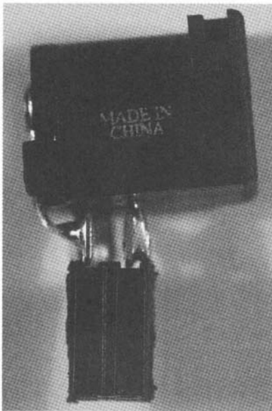
Photo 13.1: This is nothing more than a standard wall-wart power jack. I chopped off a piece of a double-row header and attached it to the power jack across two pins on each side. Pins 1 and 3 (right) are grounded while pins 2 and 4 (left) are positive voltage (+3.3 VDC). And yes, each and every one of these in that 1,000-piece bag is marked "MADE IN CHINA." Amazing, isn't it?
