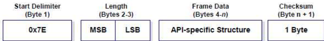
FIGURE 4-2 : UART data frame structure [19]
