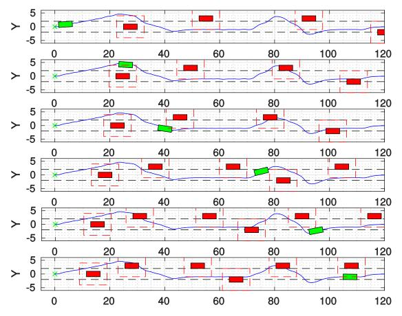
**Figure 4.9:** Simulation of overtaking with six moving obstacles that moves in the opposite direction with respect the vehicle.
