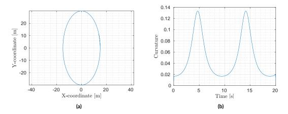
Figure 5.9: Desired elliptic path and its curvature of the ATLASCAR2 in a simulation of  $20 \, s$  with initial position in (0, 30).
