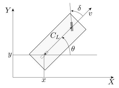
Figure 4.2: Bicycle model of a car (adapted from [37]).
