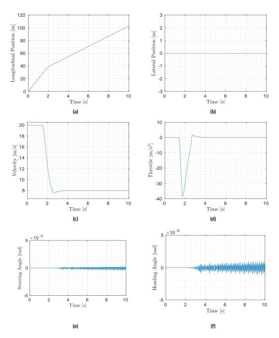
**Figure 4.12:** Time signals of the ATLASCAR2 in the simulation of no overtaking with three moving obstacles illustrated in Figure 4.11.
