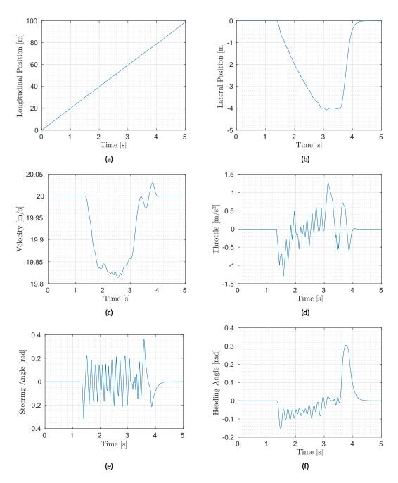
**Figure 4.7:** Time signals of the ATLASCAR2 in the simulation of right overtaking of one moving obstacle illustrated in Figure 4.6.
