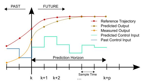
Figure 3.1: A discrete Model Predictive Control scheme adapted from [36].
