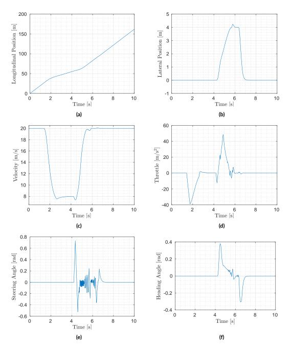
**Figure 4.14:** Time signals of the ATLASCAR2 in the simulation of braking and overtaking in the situation illustrated in Figure 4.13.
