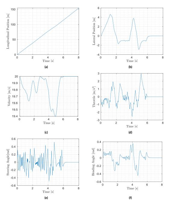
**Figure 4.10:** Time signals of the ATLASCAR2 in the simulation of overtaking with six moving obstacles illustrated in Figure 4.9.
