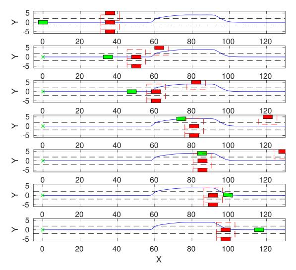
Figure 4.13: Simulation of braking and overtaking obstacles.
