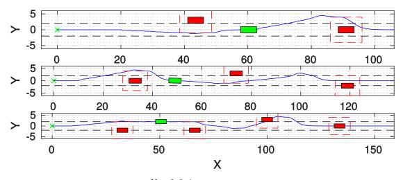
Figure 4.8: Simulations of overtaking with N = 2, 3, 4 moving obstacles that drive in the opposite direction with respect to the ATLASCAR2.
