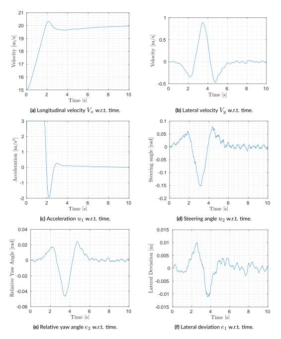
Figure 5.6: Time signals of the ATLASCAR2 in the simulation with a double lane change path.
