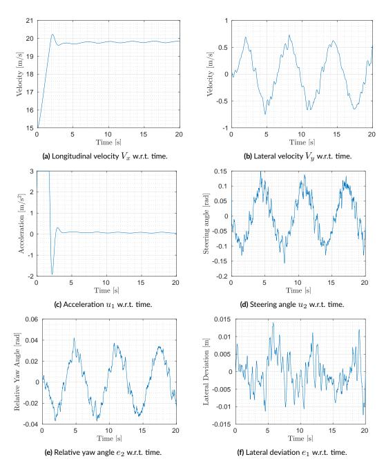
Figure 5.8: Time signals of the ATLASCAR2 in the simulation with a sinusoidal path.
