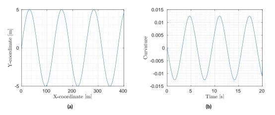
Figure 5.7: Desired sinusoidal path and its curvature of the ATLASCAR2 in a simulation of  $20\,\mathrm{s}.$
