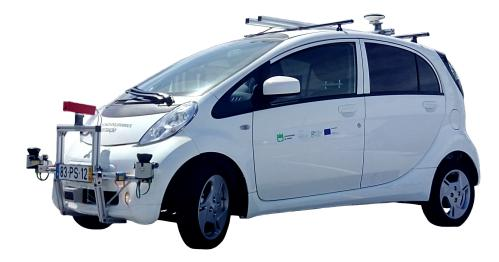
Figure 1.3: The vehicle used in ATLASCAR2, based on an electric car, a Mitsubishi iMiEV of 2015 (adapted from [11]).
