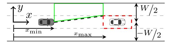
Figure 4.4: Constraints in the case of left overtaking.
