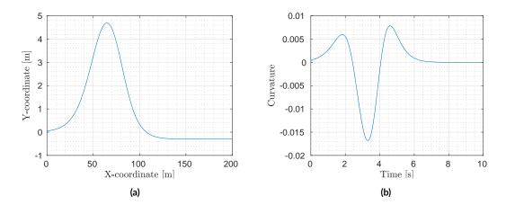
Figure 5.5: Desired double lane change path and its curvature of the ATLASCAR2 in a simulation of  $10 \, s$  with initial position in (0, 0).
