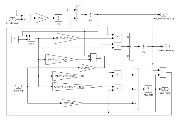
Figure 5.3: Vehicle Dynamics of the overall scheme lane following.
