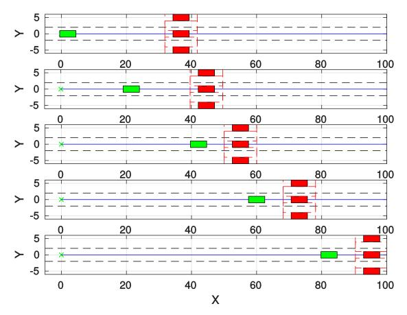
Figure 4.11: Simulation of no overtaking with three moving obstacles that move in the same direction as the vehicle.
