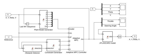
Figure 4.5: Overall procedure scheme moving obstacle avoidance.
