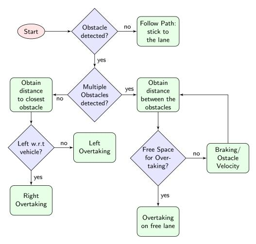
Figure 4.3: Behaviour planning conditional flowchart.
