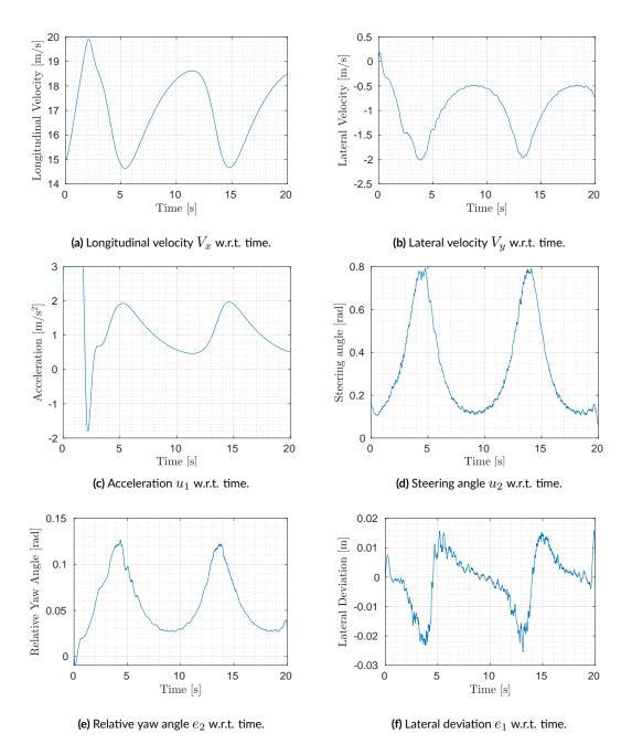
Figure 5.10: Time signals of the ATLASCAR2 in the simulation with an elliptic path.
