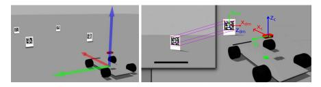
Figure 1: Navigation system through the detection of visual encoded landmarks using trilateration and related techniques [4].
