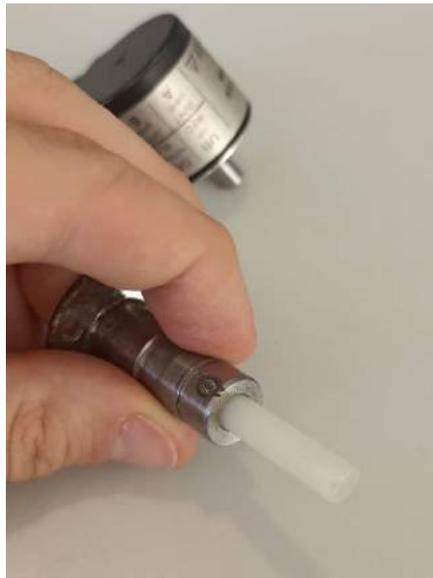
Figure 5.6: The tube that connects the encoder to the manufactured parts.
