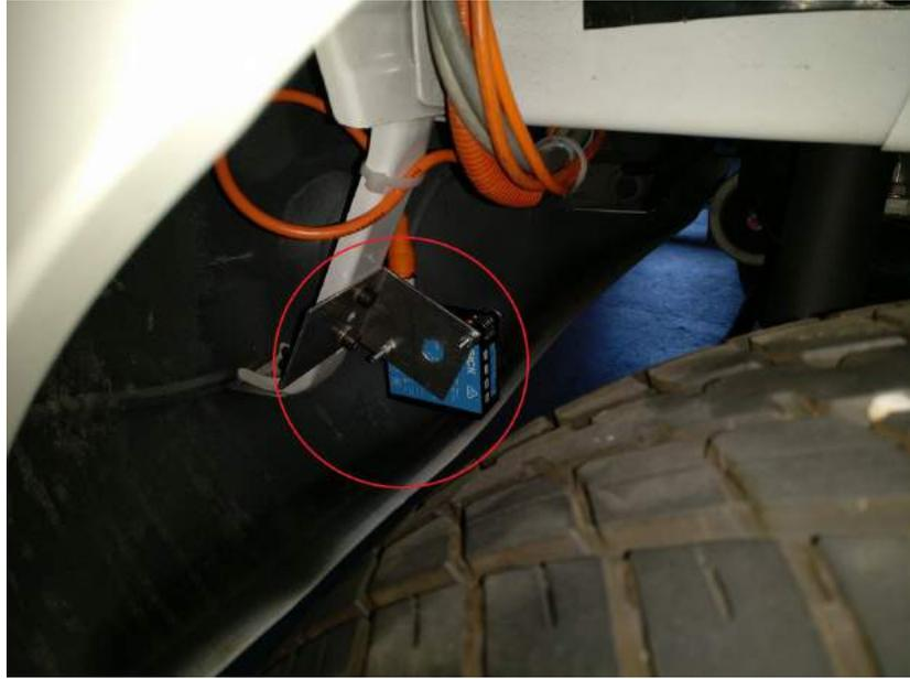
Figure 5.10: Sick DT20 Hi optoelectronic back path [74].
