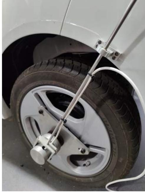
Figure 5.9: Encoder assembly in the Atlascar2.
