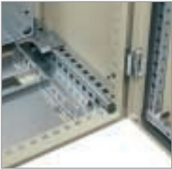
4 Guides with perforations every 25 mm to facilitate depth adjustment of the plate.
