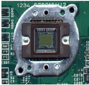
Figura 7 - CCD (charge-coupled device)
