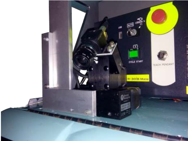
Figure 3.3: Final camera setup used to implement the navigation algorithm. Detailed view of the camera mounted on the PTU.
